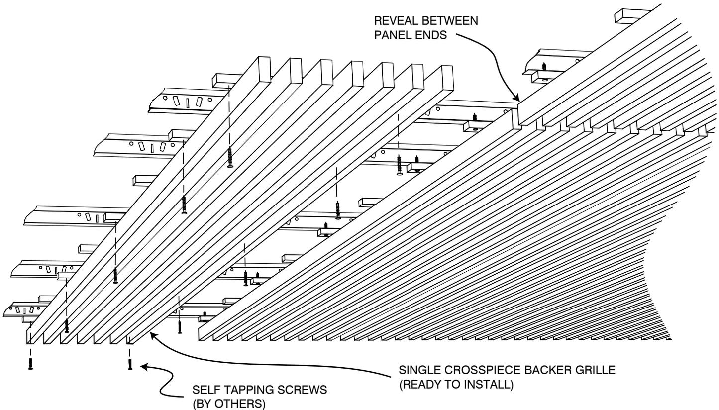
The **9Wood Dowel/Cross Piece Grille** wood ceiling offers a design where the individual wood member is deeper than it is wide. Panel width is typically 12", with backers direct-attached to T-Bar main runners every 2'. See page 3 for typical member sizes and SKUs.
