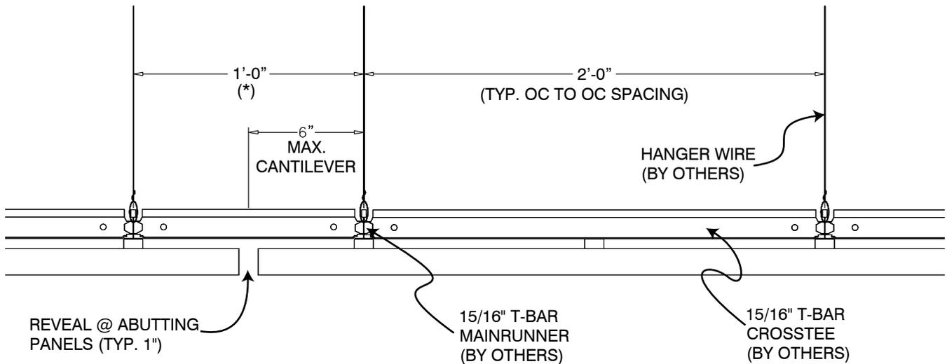
(\*NOTE: A CENTER REVEAL TYPICALLY REQUIRES A CUSTOM OC SPACING IN THE SUSPENSION SYSTEM.
